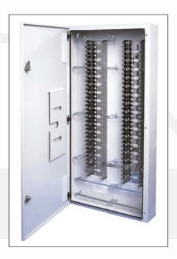
The 500 Series connection box range offers increased pair capacity whilst maintaining an industry standard footprint. The stainless steel back mount frame verticals support industry standard 10 pair disconnection strips (aka 237A). The doors can be removed entirely using quick release hinges and they can be reversed for left-right opening applications.
