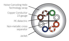
Atlas-X1<sup>™</sup> Cat 6A UTP cable features Leviton patented Noise-Canceling Helix Technology (NcHT) for superior alien crosstalk (AXT) suppression. This innovative NcHT isolation wrap also eliminates the need for grounding and bonding, saving time during installation and significantly reducing labor costs.
